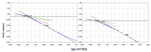
FIGURE 3: Strain-load curve, expressed as void relation, obtained on A horizon (100 to 200 mm of depth). a) soil sample 1; b) soil sample 2
