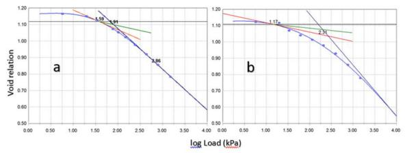
FIGURE 4: Strain-load curve, expressed as void relation, obtained on Bt1 horizon (300 to 400 mm of depth). a) soil sample 1; b) soil sample 2
