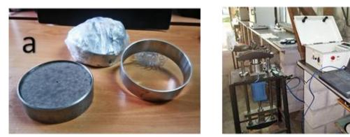
Figure 2: a) Stainless steel hoop cores, a soil sample and a soil sample as is brought from field test, before flushing. b) Uniaxial compression apparatus.
