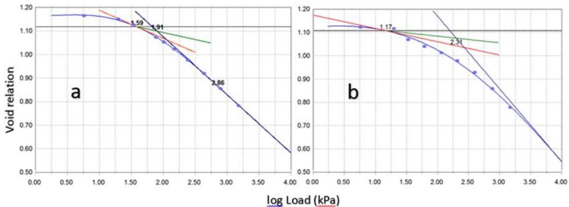
FIGURE 4: Strain-load curve, expressed as void relation, obtained on Bt1 horizon (300 to 400 mm of depth). a) soil sample 1; b) soil sample 2
