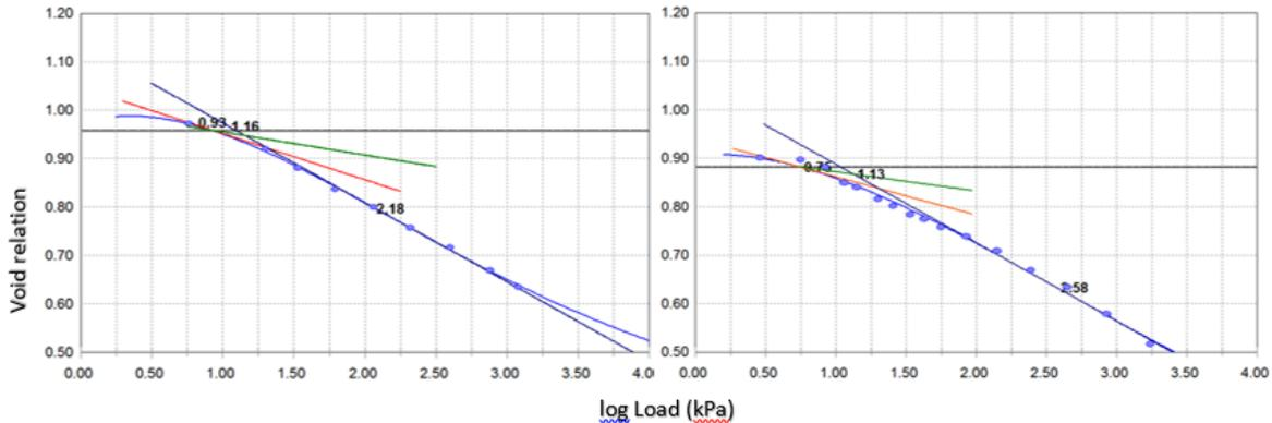
FIGURE 3: Strain-load curve, expressed as void relation, obtained on A horizon (100 to 200 mm of depth). a) soil sample 1; b) soil sample 2
