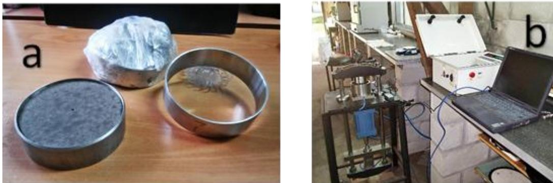
Figure 2: a) Stainless steel hoop cores, a soil sample and a soil sample as is brought from field test, before flushing. b) Uniaxial compression apparatus.
