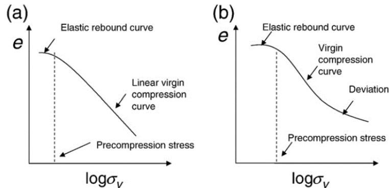
Figure 1: principal shapes of strain-load curves: bi-linear (a) and S-shaped curves (b).
