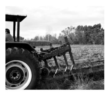
Figure 1. Experimental prototype unit for deep strip-tillage.
