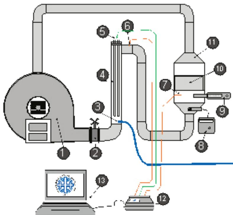
**Fig. 1.** Experimental drying equipment. 1: Fan. 2: Air velocity control. 3: Humidifying air circuit. 4: Electric heat exchanger. 5: Power electric heating regulator. 6: Air dry bulb temperature sensor. 7: Dry bulb temperature sensor in the drying chamber inlet. 8: Anemometer. 9: Hygrometer. 10: Device with sample tray holder. 11: Drying chamber. 12: Data logger. 13: Computer.
