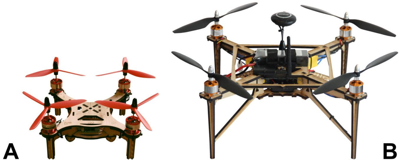
Fig 1. The Flone and OVLI drones. (A) original “Flone” design [28] upon which further versions of the open hardware drone were developed. (B) the “OVLI” drone that was developed as part of the Open Science Drone Toolkit.
