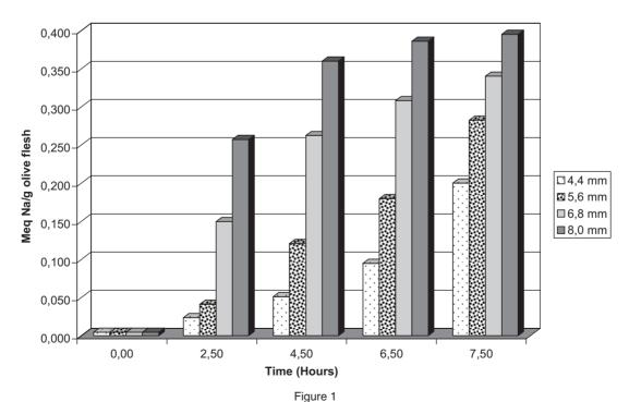
Concentration of sodium within the olive flesh during the debittering process. (Shown distances are from the pit outward).
