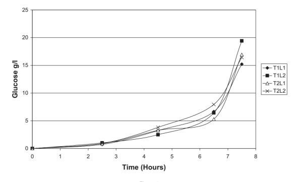
Figure 9 Loss of reducing sugars into the lye during debittering. T: represent tank and L : depth level within each tank.
