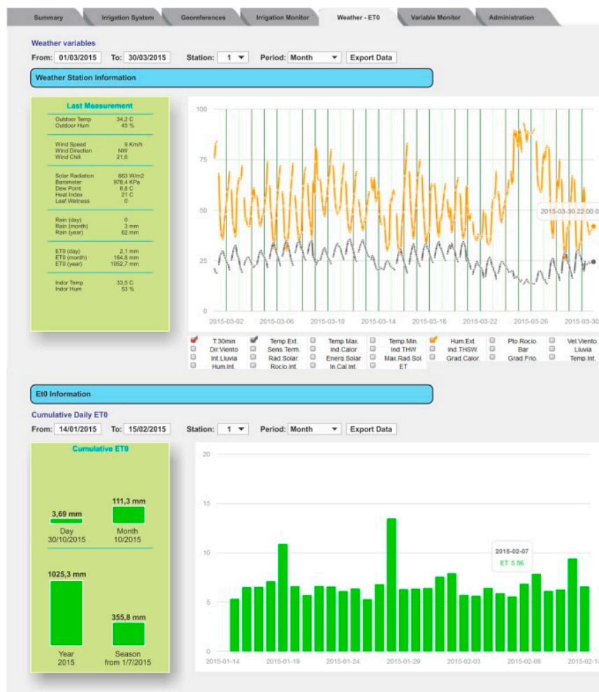
Figure 7. The Weather- ET_0 tab displays the evolution of the weather variables and the cumulative daily ET_0 estimation.
