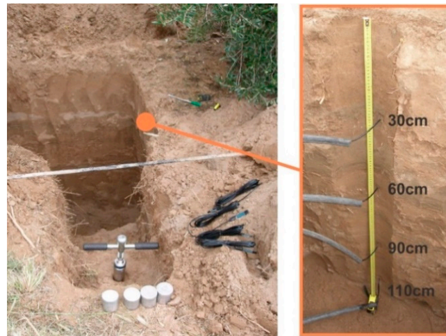
Figure 12. Soil pit performed to install four soil moisture sensors, model EC-5 from Decagon. Ten soil pits like this were made to install sensors and extract soil samples.
