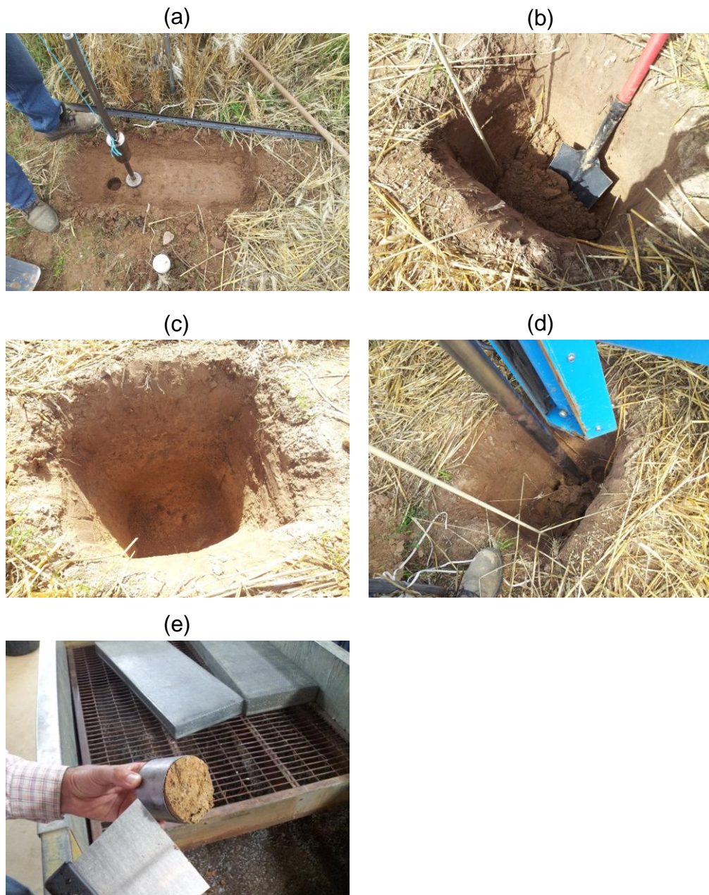
Figure 3.1. Procedures followed to sample bulk density. For the top 60 cm layers, a hand corer was used, which allowed more cautioned sampling in those layers that are more prone to crumbling (a). We dug with a shovel between sampling layers 20, 40 and 60 cm depth, avoiding compaction of the soil to be sampled (b, c). For soil layers deeper than 60 cm, we cored with the same hydraulic corer as described for sampling roots, where the coring tube was actually wider (6.5 cm diameter) (d). After removal from the soil, soil samples were levelled with a scraper in order to have a precise, known volume (e).
