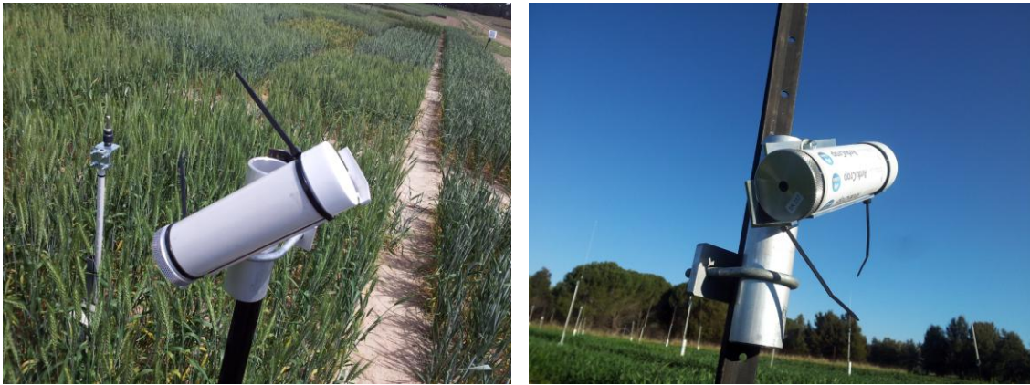
Figure 5.1. Pictures showing the infrared thermometers used to measure canopy temperature hour after hour. On the left, it can be better appreciated that they were positioned in a 45° angle from the vertical line. On the right, it can be seen more about its construction: a PVC tube inside which the electronic components are installed, and a frontal aluminium head with a hole in the middle where the infrared sensor lays.
