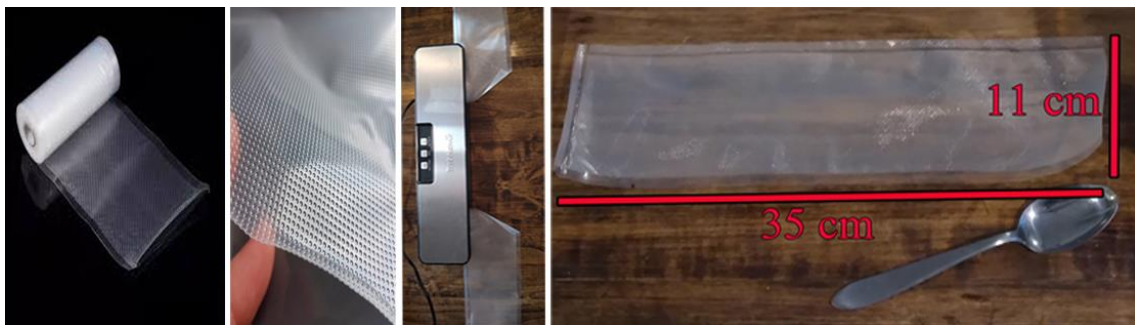
Figure 3. Embossed nylon. Edge sealing and embossed bag dimensions.
