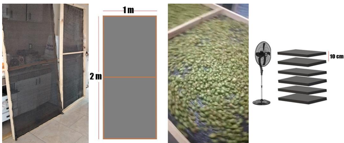
Figure 1. Drying cones: dimensions and arrangement of trays.
