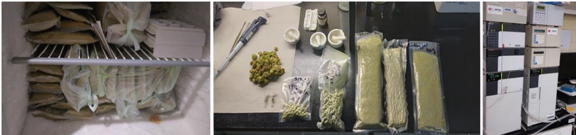
Figure 6. Storage in freezer. Measurement of alpha and beta acid content by HPLC.
