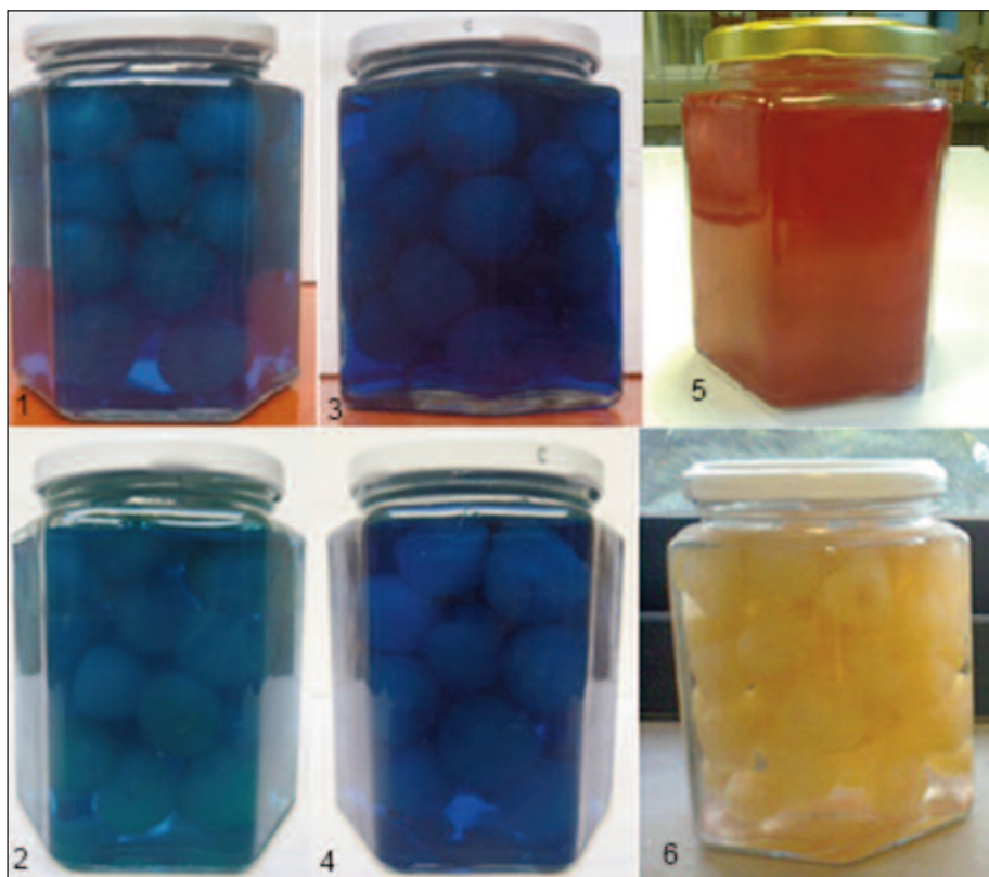
1- T3 Light Blue Brilliant before life test. 2- T3 Light Blue Brilliant after life test. 3- T2Dark Blue Brilliant before life test. 4- T2Dark Blue Brilliant after life test. 5- T1 ErB before life test. 6- T1ErB after life test.
