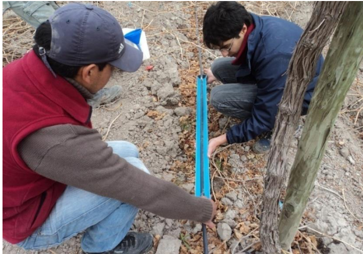
Figura 10. Volumen colectado por dos emisores en simultáneo durante 3 minutos Figure 10. Volume collected simultaneously by two emitters during 3 minutes of flow
