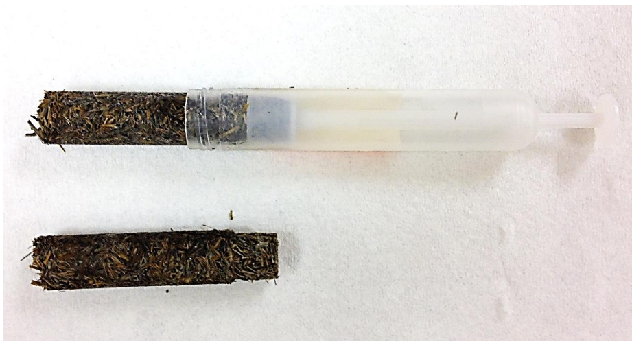
Figure 8.3 Frozen pellets containing neutral detergent fibre (NDF) from oaten hay mordanted with chromium (2.5 g of mordanted NDF, 149.5 mg Cr/pellet)
