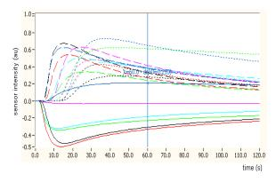
**Fig. 1.** Signals of the 18 semi-conductor metallic oxide sensors with pure and doped semiconductor.
