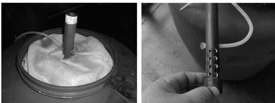
FIGURE 2. Images of the aeration system used.
