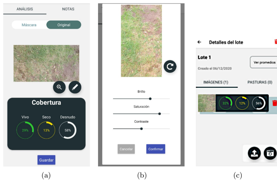
Fig. 5: Three views related to photo processing. (a) Results obtained after processing a photo. (b) One of the functionalities offered is to be able to adjust certain parameters of the image. (c) Detail of Lot 1.
