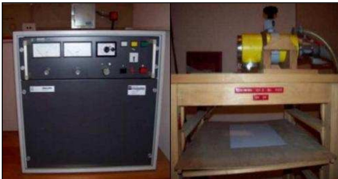
Figura 8: Irradiador de rayos X. “Philips MG-160”, Constant Potential X-Ray System (Minus H: T Generator type 160 kv 4kw)
