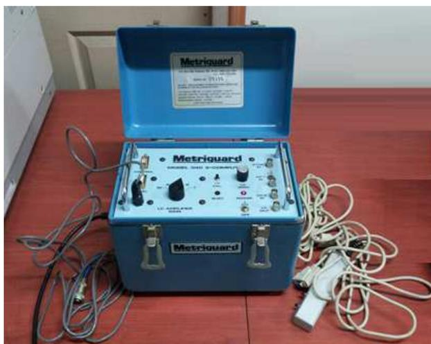
**Figura 12: Metriguard® Modelo 340 E-Computer. Tomada de Metriguard, 2002 (136).**
